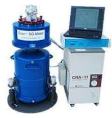
Super stable: Drift less than 0.5  $\mu$ Gal/month Scale factor constant to better than 1 part in 104 for years!
